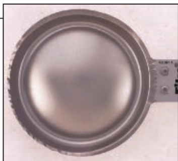
FIGURE 4. Wrinkles on the outer edge of a rupture disc indicate slippage from uneven torque
