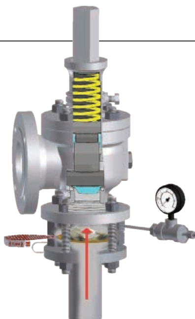
FIGURE 2. When rupture disks are used to isolate safety relief valves, the rupture disk is first to open in the event of system overpressurization. The vented process fluid then contacts the safety relief valve, which releases the fluid if the pressure is excessive
