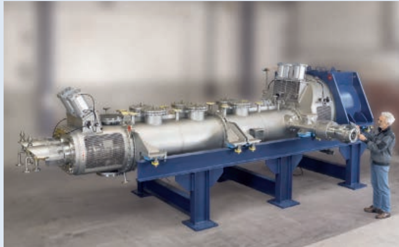
Fig. 2: Top left, Single Shaft LIST CBP KneaderReactor; Top right: Twin Shaft LIST CONTI KneaderReactor for HMM Synthesis
