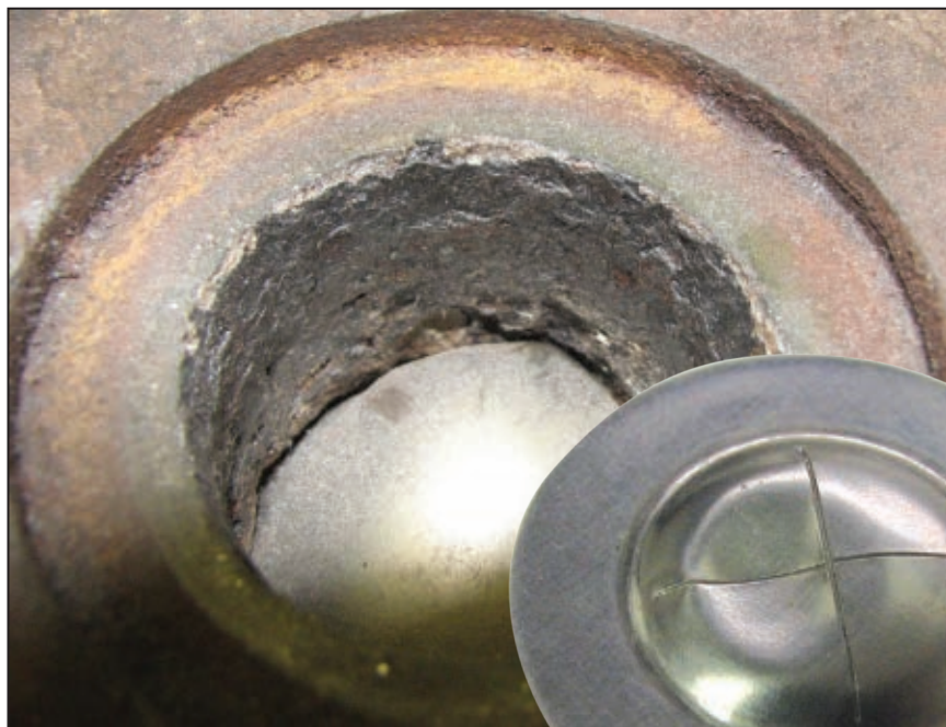
FIGURE 2. This rupture disc holder has been subjected to heavy corrosion
