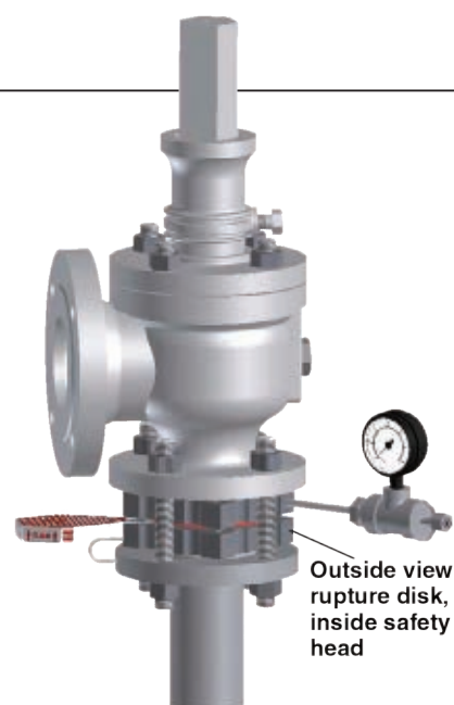
FIGURE 3. A rupture-disk and relief-valve combination will be the unrivaled choice when a leak-tight seal is needed because the system contains a corrosive, hazardous or expensive substance
